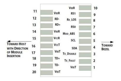
Pin-out of connector Block on Host board
