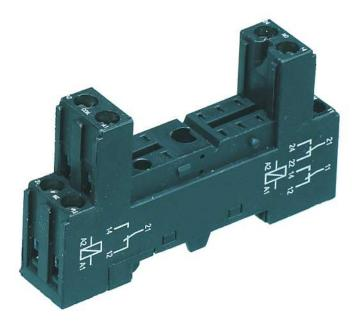
Relay socket base PRS, for miniature power relay with 2 CO contacts, Screw connection, Plug-in option for input/suppression modules, Mounting type: Mounting rail TS 35
