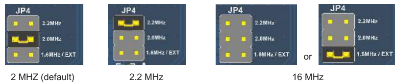
Figure 6. Switching Frequency Jumper Settings
