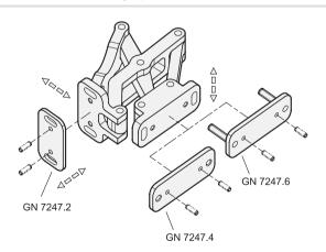
Multiple-joint hinges can be adjusted in three planes during installation. For example, this allows compensation for tolerances or establishing of required compressive forces for seals.
