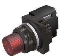
30mm BlackMax, Epoxy Coated Corrosion Resistant Complete Metal Unit Illuminated Indicator Light Full Voltage type, 6V AC/DC LED Lamp, BA9s Glass Lens, Red UL Listed, CSA Certified NEMA 1,3,3R,4,4X,12,13 & Automotive Standards
