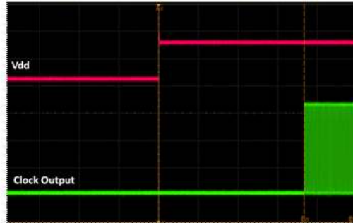
Figure 17. Startup Waveform vs. Vdd
