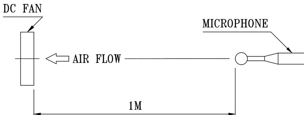
NOISE IS MEASURED AT RATED VOLTAGE IN FREE AIR IN SEMI-ANECHOIC CHAMBER WITH B & K SOUND LEVEL METER WITH MICROPHONE AT A DISTANCE OF ONE METER FROM THE FAN INTAKE.
