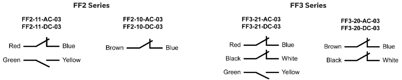
FIGURE 2. CONTACT CONFIGURATION DIAGRAMS*
