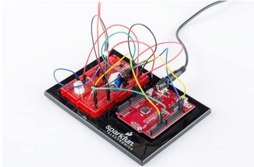
A tangled assortment of jumper wires run between the RedBoard headers and components on a breadboard. An Arduino baseplate holds them all in one place.
