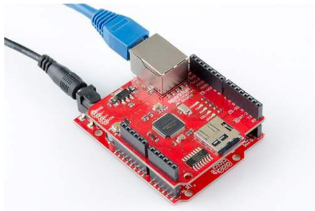
An Ethernet Shield piggybacks onto a RedBoard to help get it connected to the Internet.
