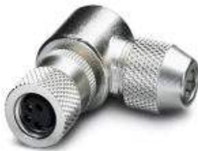
Sensor/actuator connector, socket, angled, 4-pos., M8, shielded, solder connection, metal knurl, cable diameter max. 5 mm
