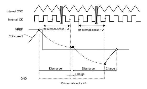
(5) Operation on change of predetermined current value (when in Charge mode)
