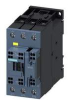
power contactor, AC-3e/AC-3, 41 A, 18.5 kW / 400 V, 3-pole, 21-33 V AC/DC, 50/60 Hz, with integrated varistor, auxiliary contacts: 1 NC, main circuit: screw terminal, control and auxiliary circuit: spring-loaded terminal, size: S2, F-PLC-IN
