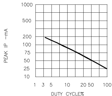
Fig.6 MAX PEAK CURRENT VS. DUTY CYCLE %
