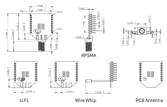
The following drawings show the XBee-PRO through-hole device.
