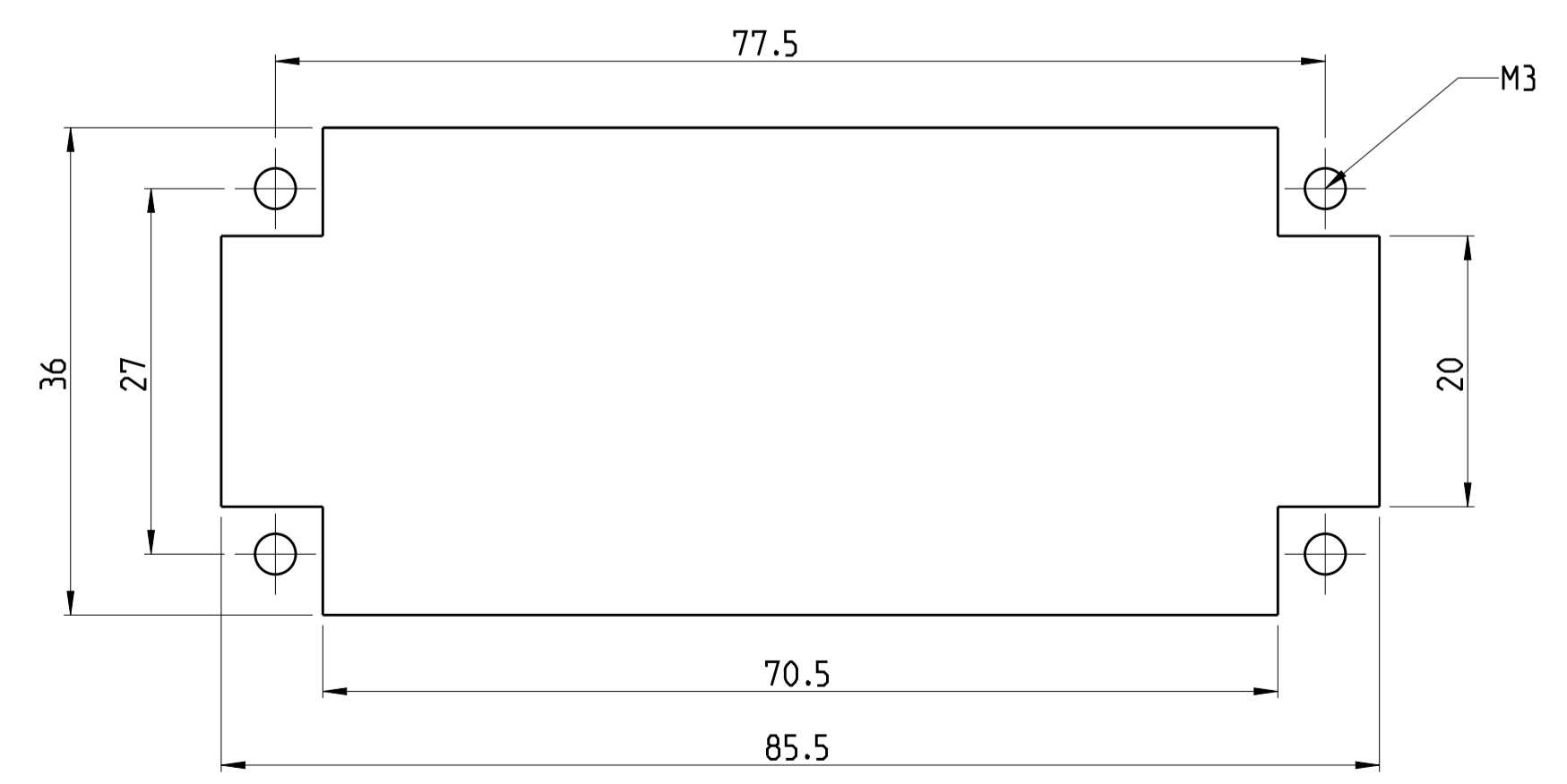
PANEL CUT-OUT FOR CONTACT INSERT WHEN USED WITHOUT HOUSING
