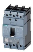
circuit breaker 3VA5 UL frame 125 breaking capacity class M 35kA @ 480 V 3-pole, line protection TM230, FTAM, In=50A overload protection Ir=50A fixed short-circuit protection li=5...10 x In cable connection on both sides
