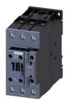
power contactor, AC-3e/AC-3, 65 A, 30 kW / 400 V, 3-pole, 200 V AC, 50 Hz / 200-220 V, 60 Hz, auxiliary contacts: 1 NO + 1 NC, screw terminal, size: S2
