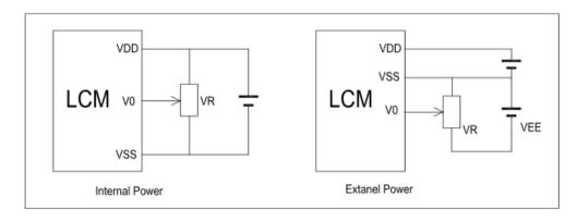
VDD-V0: LCD Driving Voltage VR: 10k-20k
