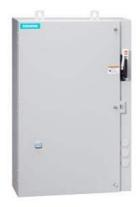
Non-reversing motor starter Size 3 Three phase full voltage Solid-state overload relay OLRelay amp range 25-100A 380-440/440-480V 50/60HZ coil Combination type 100A fusible disconnect 100A/600V fuse clip Enclosure NEMA type 4/12 Water/dust tight weather proof Standard width enclosure
