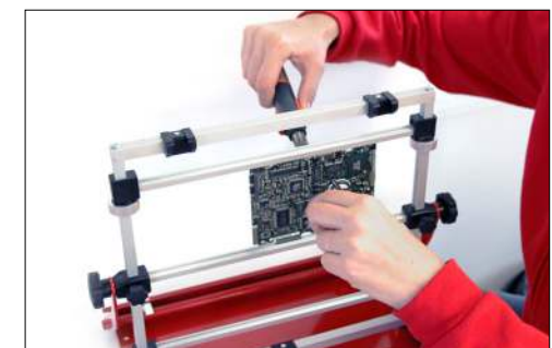
Unsoldering of components carried out with PC Assembly Jig in vertical positions.
