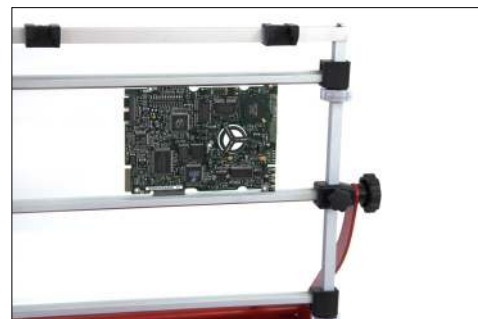
Practical use of PC Assembly Jig with PC Board in place.
