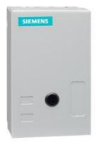
Electrically held lighting contactor, Contactor amp rating 20A, 0 N.C. / 3 N.O. Poles, 198VAC 50HZ/208VAC 60HZ coil, Non-combination type, (no disconnect device), Enclosure NEMA type 1, Indoor general purpose use
