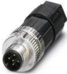
Sensor/actuator connector, male, straight, 5-pos., M12 SPEEDCON, A-coded, spring-cage connection, metal knurl, cable diameter max. 8 mm
