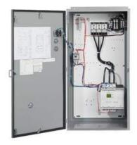
Enclosed soft starter, Controller 3RW44366BC34, Std. duty rating 75KW @380V, Std. duty current rating 145A Control voltage 115Vac Enclosure NEMA type 12, Dust/drip proof for indoors
