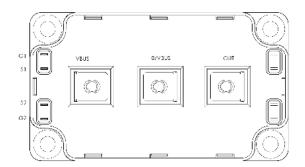
$$\begin{split} V_{DSS} &= 600 V \\ R_{DSon} &= 18 m \Omega \ max \ @ \ Tj = 25^{\circ} C \\ I_D &= 143 A \ @ \ Tc = 25^{\circ} C \end{split}$$
