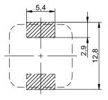
no sensitive traces underneath the component
