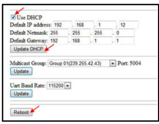
2. Set the IP Via Web Browser: When using a switch that doesn't support DHCP, change the default IP manually:
