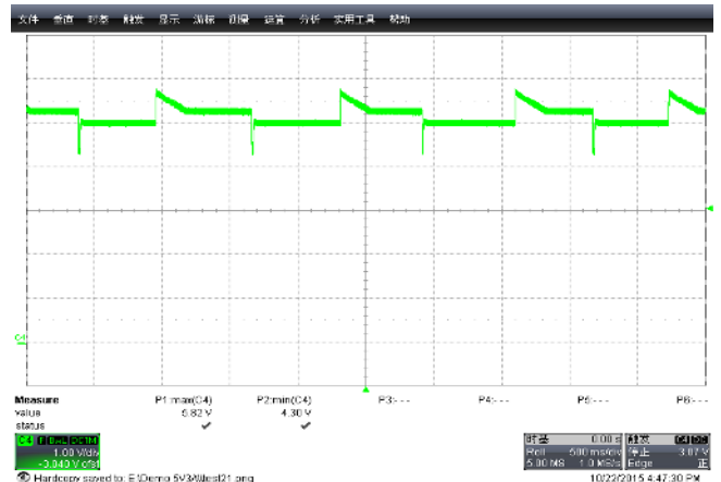
Fig:15 Vo_min=4.41V & Vo_max=5.82V at 265Vac
