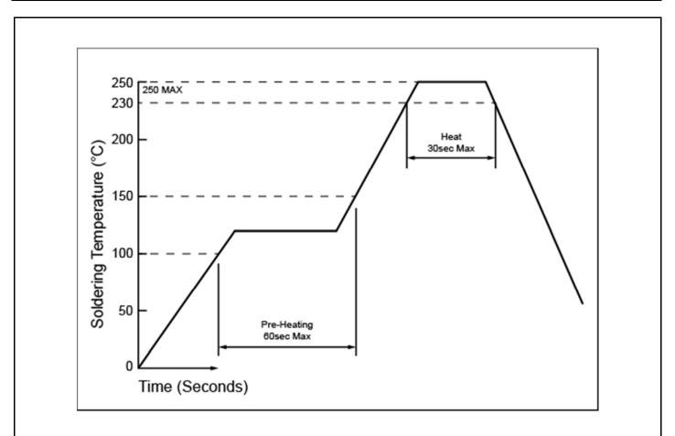
Fig. 1. Recommended Reflow Temp. Profile
