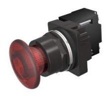
30mm BlackMax, Epoxy Coated Corrosion Resistant Complete Metal Unit Illuminated Push-Pull Operator Full Voltage, 24V AC/DC Incandescent Lamp Mushroom Head Cap Small 1 3/4" (44.5 mm) Plastic, Red 3 Position Momentary UL Listed, CSA Certified NEMA 1,3,3R,4,4X,12,13 & Automotive Standards
