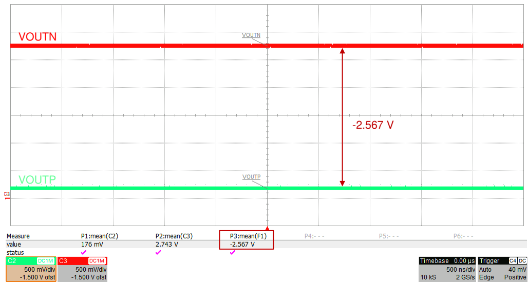
Figure 7-5. Typical Fail-Safe Output of the AMC3330-Q1
