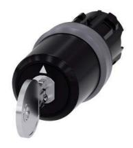
Key-operated switch BKS, 22 mm, round, plastic with metal front ring, lock number S1, with 2 keys, 3 switch positions I-O-II, latching, actuating angle  $2x45^{\circ},\,10:30h/12h/13:30h,$  key removal O, with laser labeling, lower case
