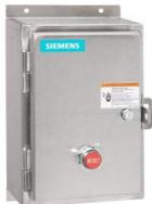
Non-reversing motor starter Size 1 Three phase full voltage Solid-state overload relay OLRelay amp range 0.75-3.4A 208VAC 60HZ coil Combination type Water/dust tight non-corrosive
