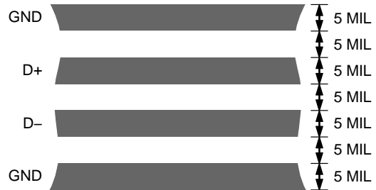
Figure 34. Typical Arrangement of Signal Tracks
