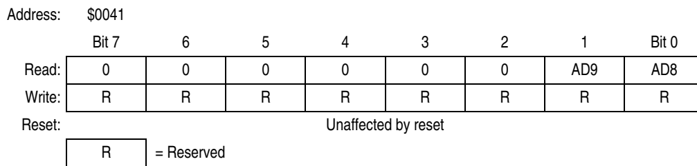
Figure 3-6. ADC Data Register High (ADRH) Right Justified Mode
