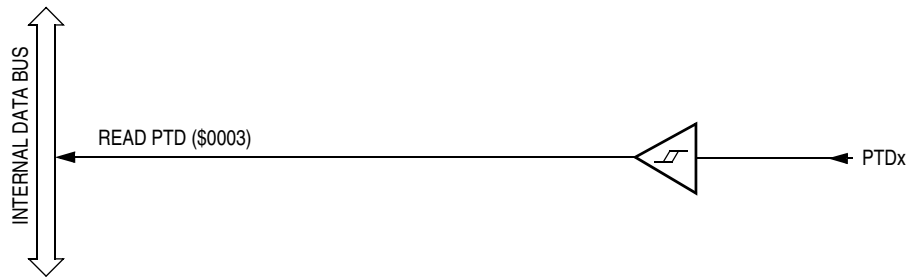
Figure 10-12. Port D Input Circuit
