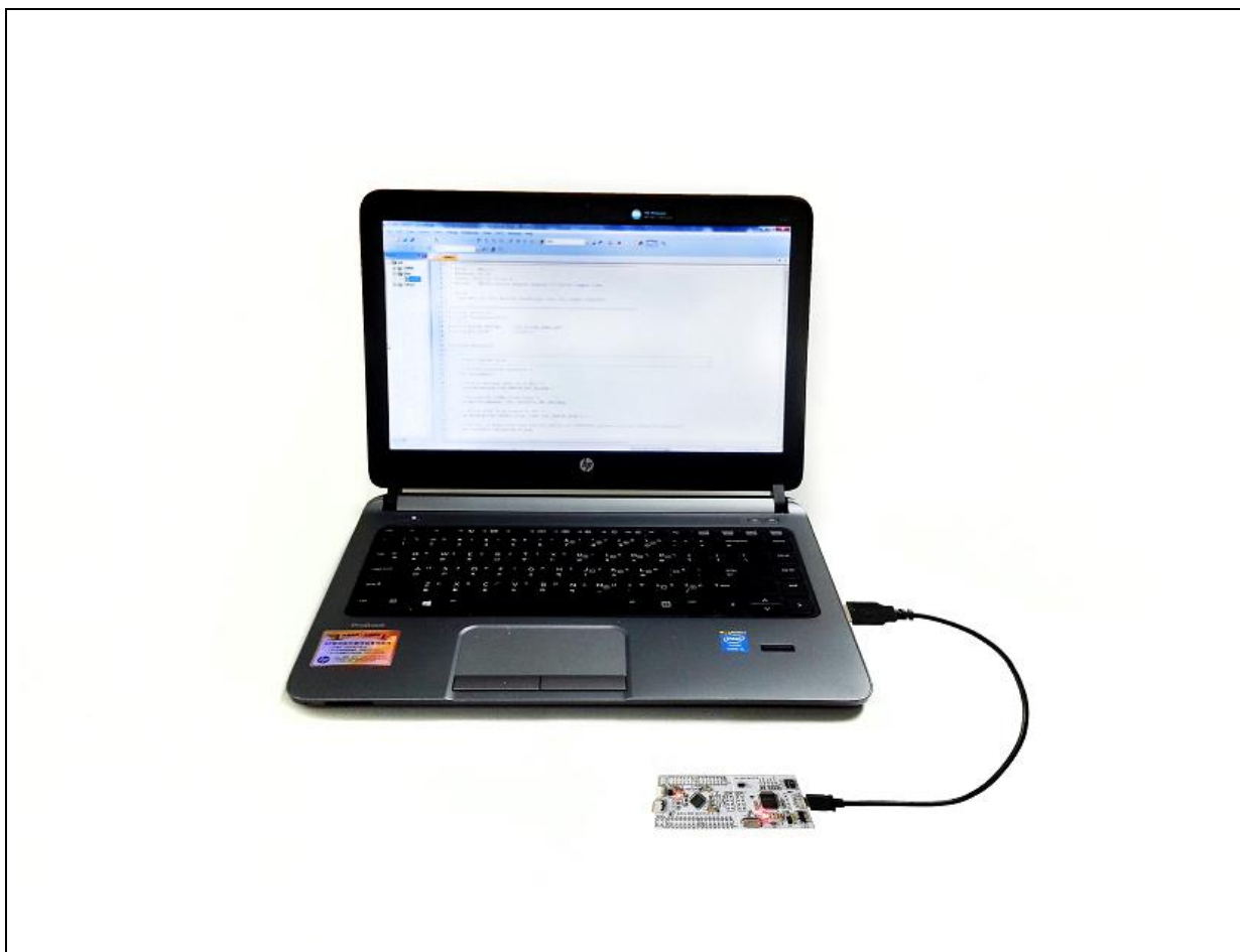
Figure 4.3-1 NuTiny-SDK-NUC121/125 Hardware Setup
