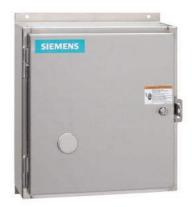
Non-reversing contactor, Size 2 1/2, Three phase full voltage, Contactor amp rating 60A, 3 wire (NO aux included), 208VAC 60Hz coil, Non-combination type, Encl NEMA type 4X 304 S-Steel, Water/dust tight noncorrosive, Extra-wide enclosure
