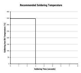
The soldering iron tip temperature should be set at 350°C (+10°C maximum) with the soldering duration not to exceed more than 3 seconds.
