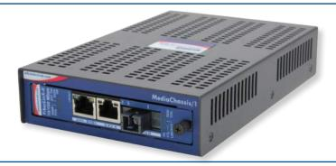
The MediaChassis/1, flexible, table-top chassis that supports a variety of B+B SmartWorx media and mode converter modules available for Fast Ethernet, Gigabit, T1/E1, DS3/E3/STS-1 and mode conversion networking technologies. This modular approach allows network operators to inexpensively change protocols by simply changing the module rather than the entire unit.
