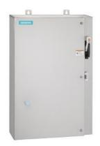
Non-reversing motor starter Size 2 1/2 Three phase full voltage Solid-state overload relay OLRelay amp range 25-100A Combination type 100A non-fusible disconnect Encl NEMA type 4X 316 S-steel Water/dust tight non-corrosive Extra-wide enclosure
