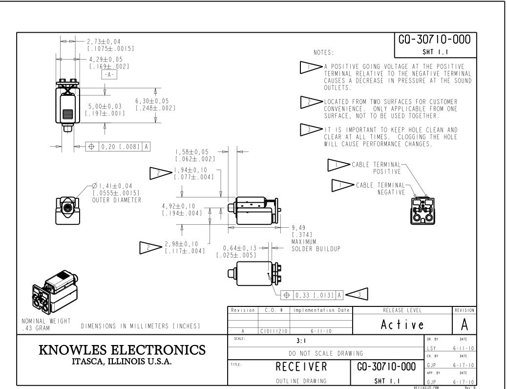
UNDAMPED MAGNETIC BALANCED ARMATURE RECEIVERS INTENDED FOR USE AS THE HIGH AND LOW FREQUENCY DRIVERS IN A HI FI SYSTEM. THE GO RECEIVER COMBINES A WBFK AND ED RECEIVERS COUPLED THROUGH A CIRCUIT TO PROVIDE THE RESPONSE SHAPE.
