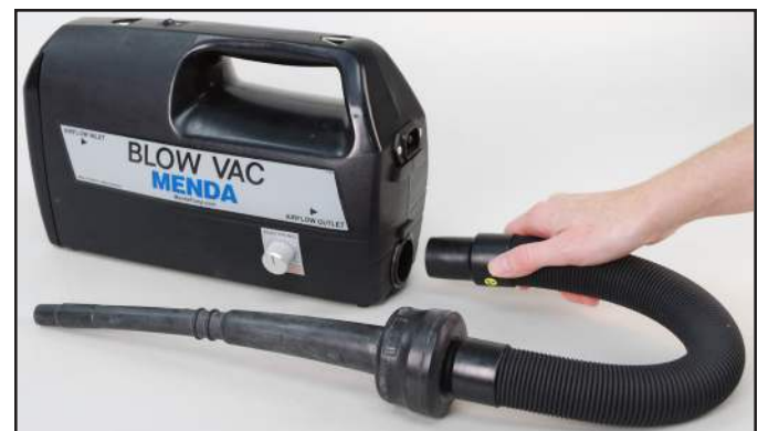
Figure 2. Connecting the hose to the airflow outlet
