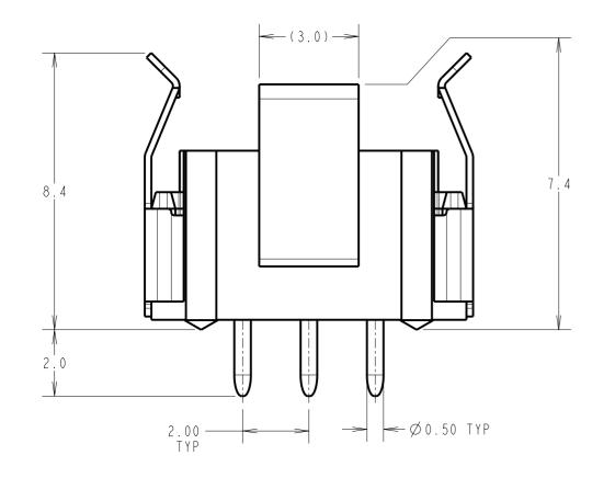
COMPONENT SPECIFICATION: MATERIAL: MOULDING: GLASS FILLED PPS, UL94V-0, BLACK CONTACT: COPPER ALLOY LATCH: BERYLLIUM COPPER P&P CAP: POLYIMIDE PA4T 30% GF TAPE: POLYSTYRENE COVER TAPE: POLYESTER FINISH: CONTACT: TIN OVER NICKEL ON TAILS, GOLD OVER NICKEL ON CONTACT AREA LATCH: NICKEL
