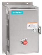
Non-reversing motor starter, Size 0, Three phase full voltage, Solid-state overload relay, OLR amp range 5.5-22A, 24VAC 50-60Hz coil, Non-combination type, Encl. type 4X 304 S. Steel, Water/dust tight noncorrosive, Standard width enclosure
