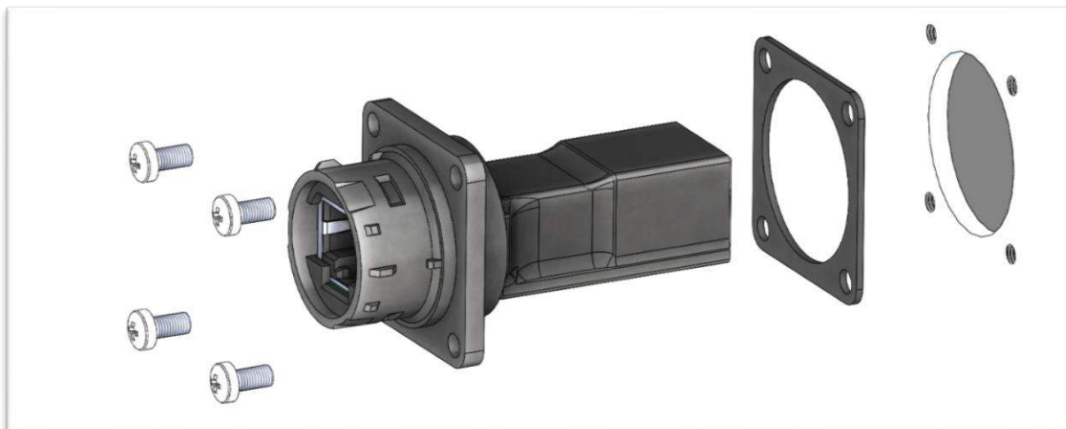
Figure 11. Assembly of EN-10HG into a housing panel opening
