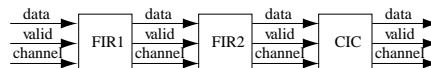
Figure 18. 16-channel WCDMA DUC Design Shows how channel's distribution on wires change in a multirate system.
