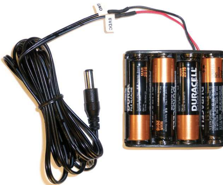
Figure 69. Recommended Power Supply for ADS1299EEG-FE
