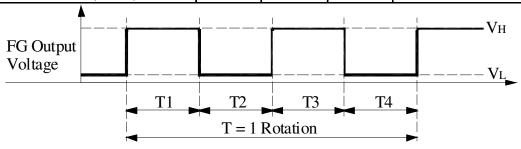
T=T1+T2+T3+T4=1 Rotation  $T=\frac{60}{\text{rpm}}$
