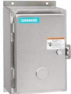
Non-reversing NEMA contactor, Size 1, Single phase full voltage, Contactor amp rating 27A, 3 wire (NO aux included), 110-120/220-240VAC 60Hz coil, Non-combination type, Encl NEMA type 4X 304 S-Steel, Water/dust tight noncorrosive, Standard width enclosure
