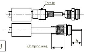
Cut the dielectric flush to crimp sleeve. Mount insulator against crimp sleeve.
