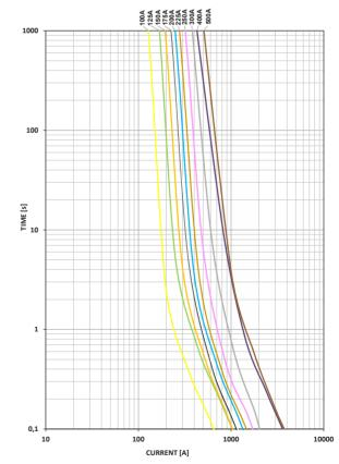
100A-300A:  $F_L$ =1,25 (max. operating current: 0,8 x  $I_{rat}$  at 23°C) 400A-500A:  $F_L$ =2,00 (max. operating current: 0,5 x  $I_{rat}$  at 23°C)
